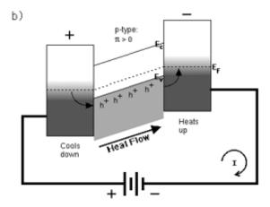
Fig4.Π>0; Positive Peltier coefficient
