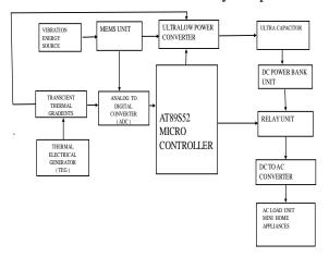
Fig6.Block diagram of hybrid power converter
