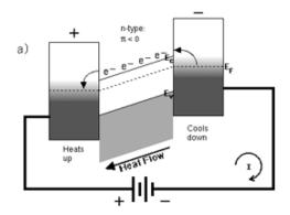
Fig3. Π<0; Negative Peltier coefficient
