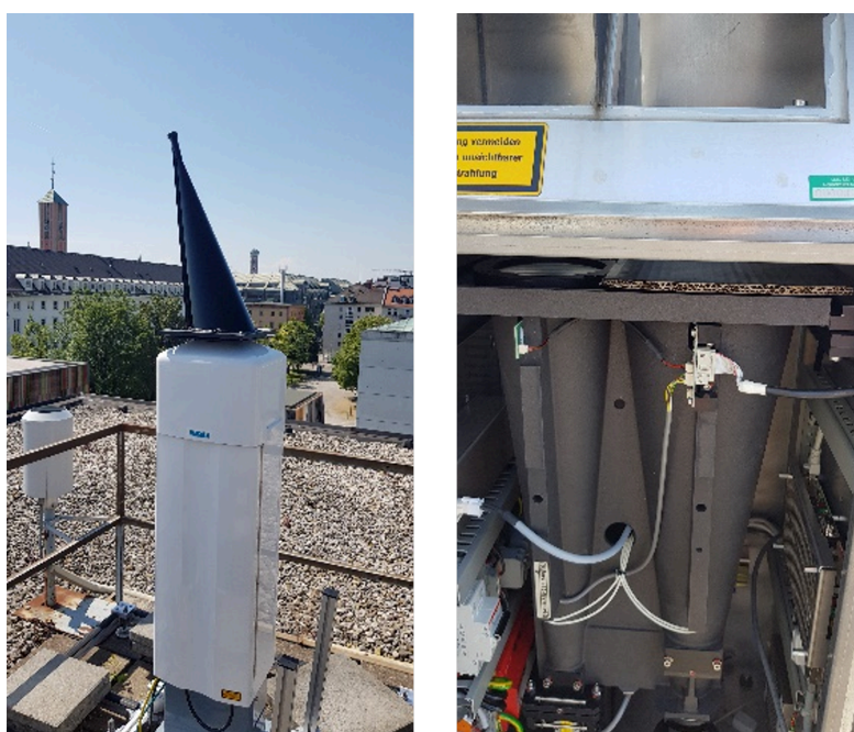
Figure 6: Vaisala CL31 (monostatic) with optical termination hood (left) and laser optical module (LOM) of Lufft CHM15kx (bistatic) with cardboard covering the telescope (right) from the ACTRIS CARS ALC unit testbed.
