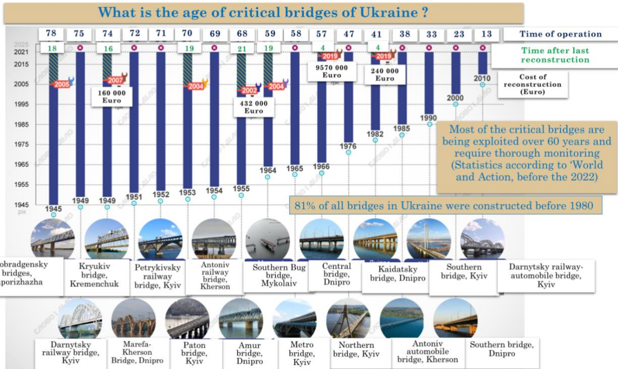
Figure 5. The issue of ageing of the most critical bridges as the part of critical transport infrastructure in Ukraine.
