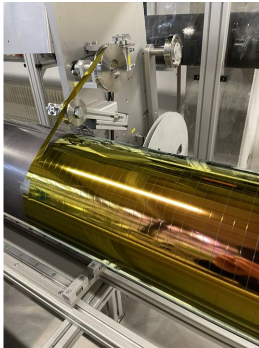
Fig. 2 roll-to-roll coating support adapted to wide tapes.
