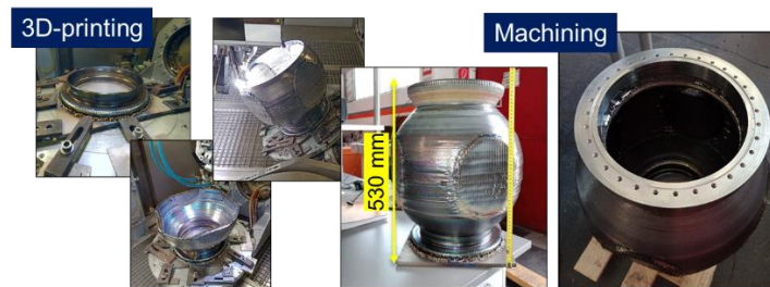
Fig. 30 Progress of vacuum chamber manufacturing.
