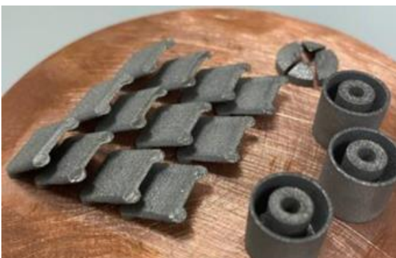
Fig. 18 Successful production of different inclined walls (top) result of the surface roughness measurement of down skin surfaces.
