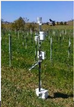
Meteorological station (rainfall, air temperature and humidity, atmospheric pressure, wind speed and direction)
