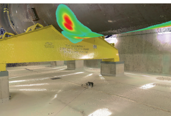
Source location: back-projection of the signal emerging from a source on the 3D topographic survey
