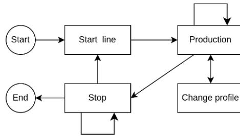
**Fig. 1** State-based model diagram of a single machine’s transitions
