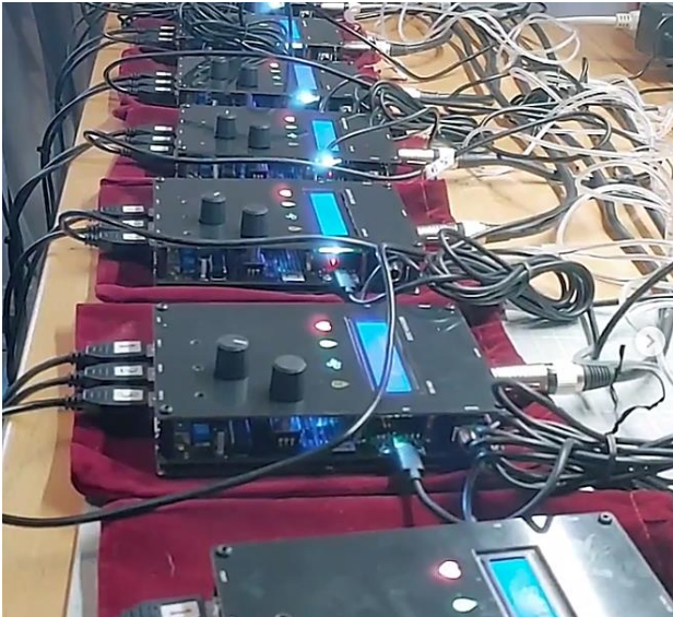
Figure 4. Several BioSynth devices connected in a modular fashion to share their power supply.
