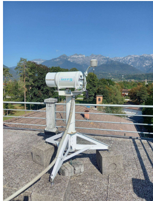
Figure 24: Example of operational MTP5-HE microwave radiometer in the ARPA Veneto profiler network. Picture provided by Massimo E. Ferrario, ARPA Veneto.
