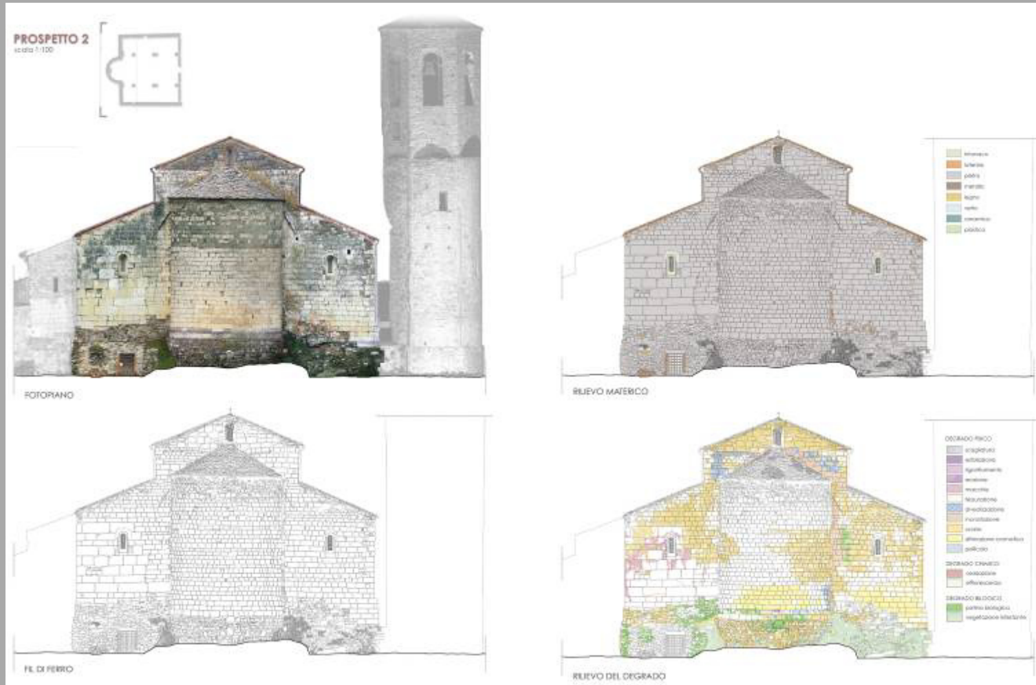
Examples of themed maps of the Pieve a Socana (AR) – From left to right and from top to bottom: orthophoto, identification of the material, CAD drawing, analysis of decay
