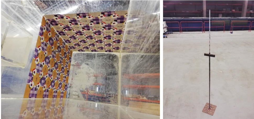
Figure 18. Targets to perform the scaling and referencing of the sediment-bed 3D reconstruction (left), and graded rod for field measurements (right).
