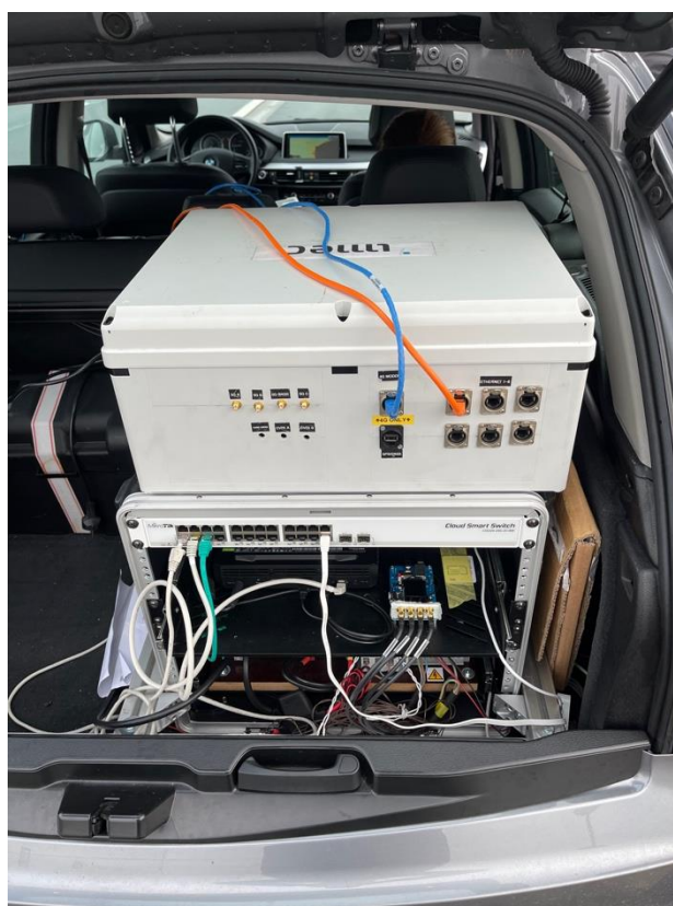
Figure 27. Box with the 5G Modem (Peplink), GPS, and camera.
