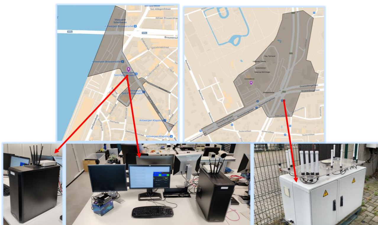
Figure 26. Open5G testbed with coverage maps.
