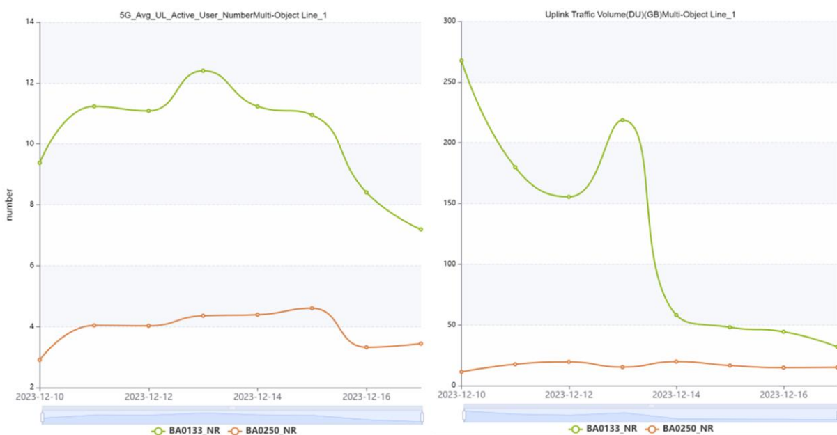
Figure 23. Measured number of users and uplink traffic at the NR gNodeB level during December tests.
