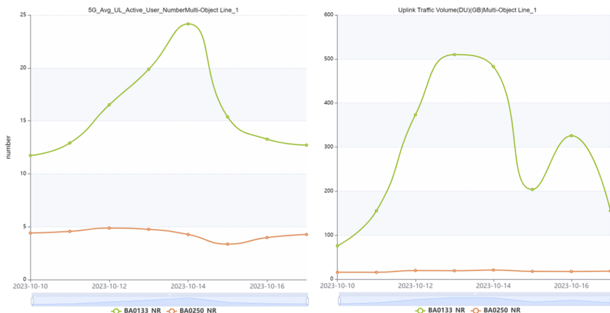
Figure 22. Measured number of users and uplink traffic at the NR gNodeB level during October tests.
