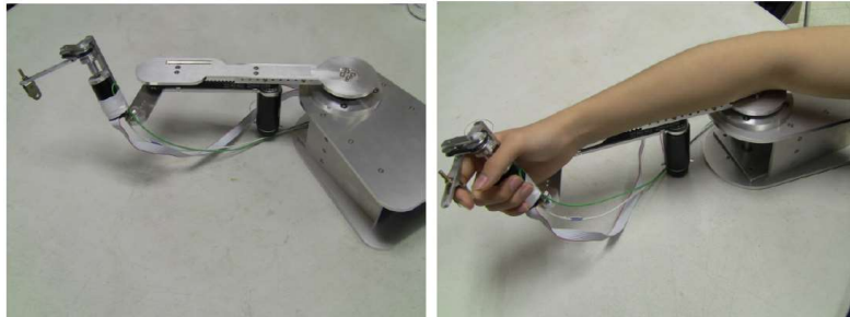
Figure 9 – New haptic interface design for the teleoperation of excavators based on their shape
