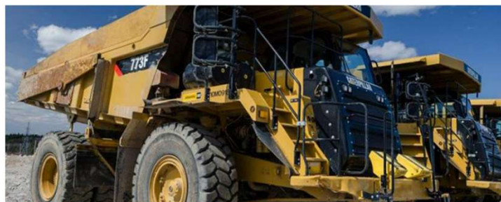
Figure 10 – Dumper 773F. It is a common machinery in the execution of large infrastructures, as it is used for moving soil. This truck is more than 4.3 meters high and more than 10 meters long and has a load capacity of 50 tons.
