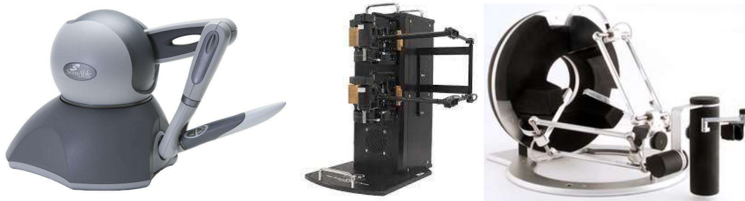
Figure 5 – Commercial examples of haptic devices. From left to right: Sensable-Phantom Omni (serial), Quanser-HD2 (parallel), ForceDimension-Omega.7 (hybrid)
