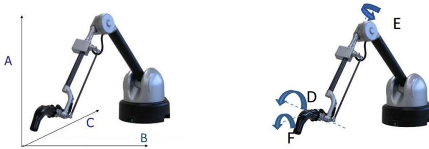
Figure 15 – Virtuose 6D haptic has 6 DoF (3 translational, 3 rotational)
