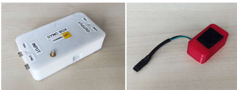
Figure 3: SyncBox (left) which reproduces an input signal on the remote trigger device (right).
