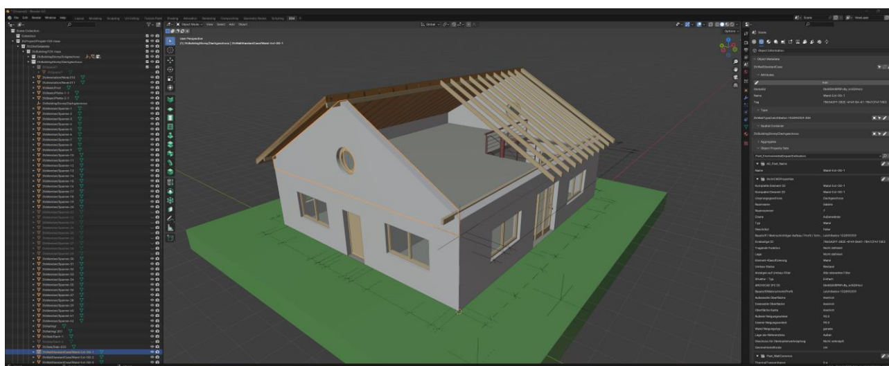
Figure 5 Overview of the BlenderBIM GUI with the IFC Entities (left), 3D Model (middle), Entity property sets (right)
