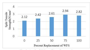
Fig. 6. Graph of 28day split tensile strength
