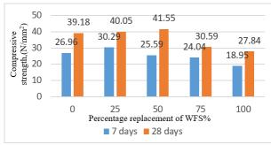
Fig. 5. Graph of 7 & 28days compressive strength
