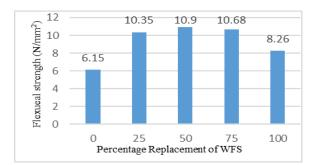
Fig. 7. Graph of 28day flexural strength test
