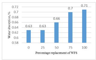
Fig. 10. 28days water absorption of beam
