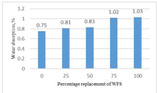
Fig. 9. Graph of 28days water absorption of cylinder
