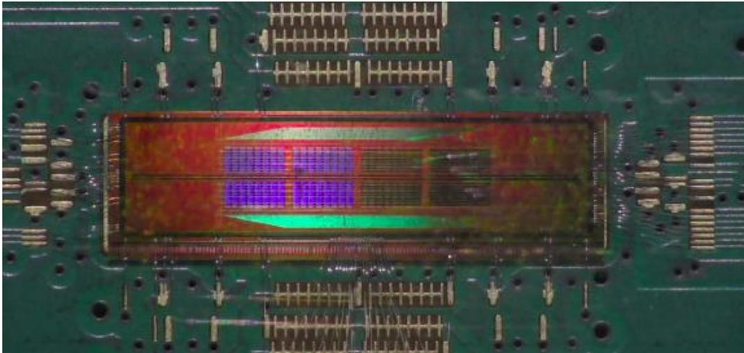
*Fig. 2: Photograph of the ARCADIA MADPIX prototype mounted on a readout board.*
