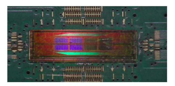
Fig. 2: Photograph of the ARCADIA MADPIX prototype mounted on a readout board.
