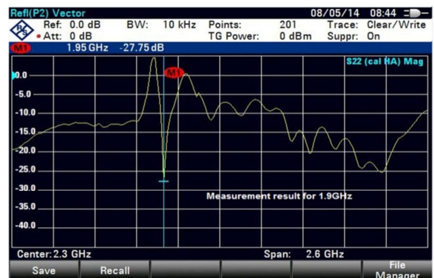
Fig. 4 (b) Measured result of output return loss at the frequency of 1.9 GHz
