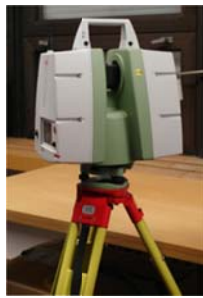
Fig. 1 Spatial scanner Leica ScanStation C5
