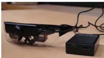
Fig. 5 The augmented reality glasses Vuzix STAR 1200XLD
