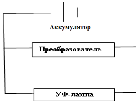
Figure 1. Scheme of irradiation of cotton with ultraviolet rays
