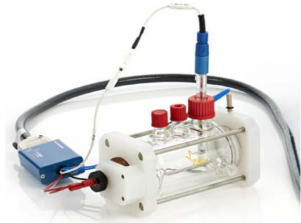
Fig. 3 Three electrode corrosion cell (capacity 300 cm 3 )
