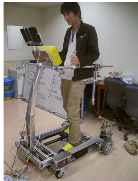
Fig. 2 Rehabilitation center training robot for basic walking-pattern training. The robot has two motors for the two sliding mechanisms, two motors for maneuvering on the floor, and two kinds of pressure sensors on the steps, and touch switches on the step covers
