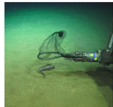
Figure 31. ROV SuBastian expertly manipulating a hand net to capture a fish. Photo SOI.
