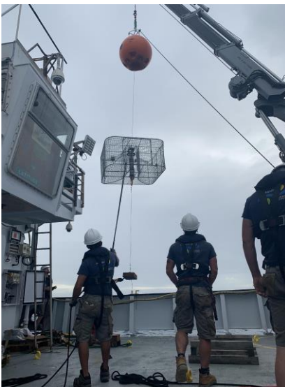
Figure 26. Large fish trap being deployed by deck crane with a syntactic float. Photo SOI.
