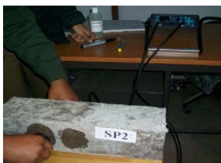
Fig. 9 Typical locations of transducers on the specimen
