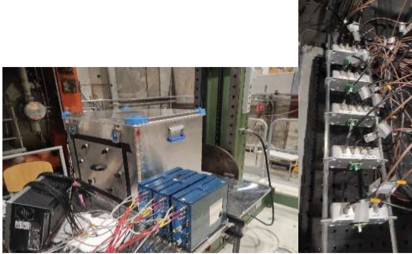
Figure 11: Photos taken during the 2023 test beam campaign. The image on the left features the dark-tight box containing the samples with three DWCs in front. On the right, the picture depicts the samples connected to their respective readout boards, shielded by a metal case.
