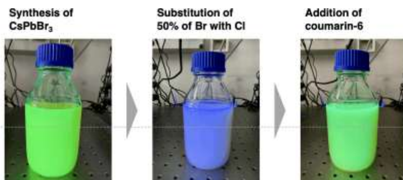
Figure 20: Preparation of monomer solution for nanocomposite with caesium lead halide perovskite with coumarin-6 WLS.
