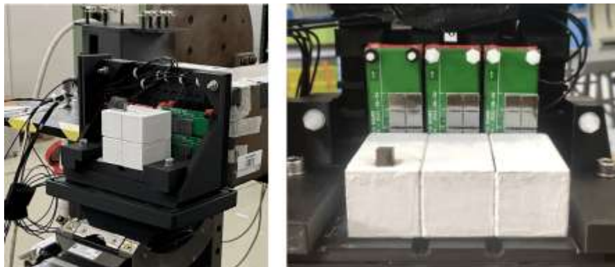
Figure 18: 2 \times 2 and 1 \times 3 assemblies of crystals with pre-alignment of crystallographic axes during the summer 2023 beam tests. A silicon mirror used to provide an absolute angular reference for the whole assembly is visible at the upper left in each case.
