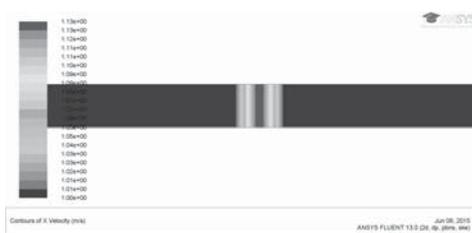
Fig. 3. Contours of X velocity, RANS
