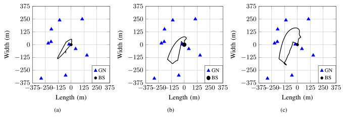
Fig. 7: Optimal UAV trajectories: (a)  $B_c = 30$  Wh (b)  $B_c = 45$  Wh (c)  $B_c = 60$  Wh.
