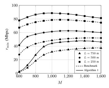
Fig. 3: Minimum rate vs the number of reflecting elements M for  $\sigma^2 = -144$  dB.
