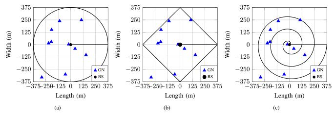
Fig. 2: Benchmark UAV trajectories: (a) Circle (b) Rombus (c) Spiral.
