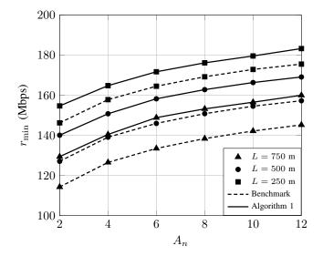
Fig. 4: Minimum rate versus UAV-mounted FDR Antennas for  $\sigma^2 = -144~\mathrm{dB}$
