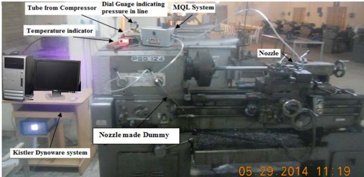
Fig. 1 Experimental set up with Coolubricator system
