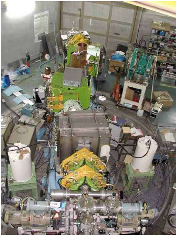
A recoil mass separator consisting of QQEMDDQQ (upper part) and a windowless gas target (lower part) for astro-nuclear experiments.
