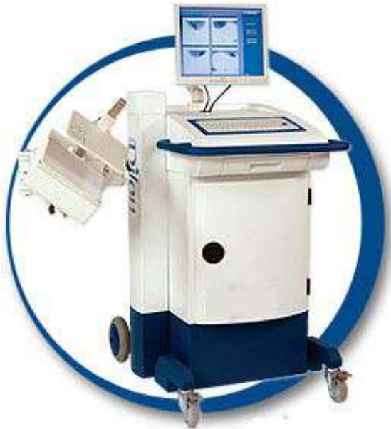
Nuclear techniques have transformed medical imaging, as illustrated here by the Dilon Gamma Camera, used in the scanning for breast cancer.
