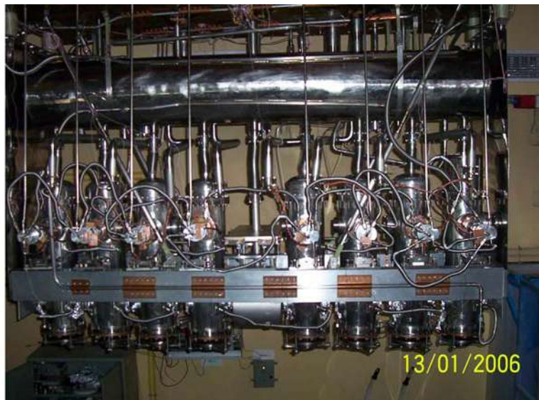
Figure 1. Arrangement of the QWR cavities in the first Linac module.
