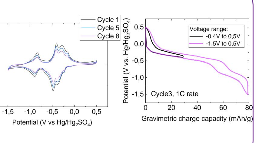
NFP was cycled at 1C in voltage range -0,4V to 0,5V and -1,5V to 0,5V. Capacity differs depending on the voltage range (close to 97 mAh/g in the wider voltage window).
