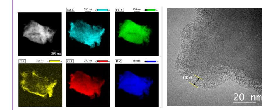
TEM analysis was done Na<sub>2</sub>FeP<sub>2</sub>O<sub>7</sub> for raw powder. Obtained show clearly images carbon coating with thickness fluctuating from 3 to 9 nm. Carbon coating is in part amorphous and in part graphitic.
