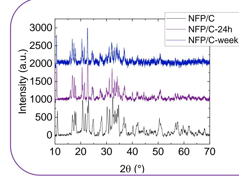
Stability of NFP/C in water was tested by immersion in water for 24h and 7 days. The XRD data of the subsequently dried samples is shown in the graph.
