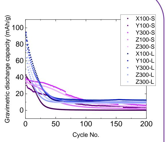
S (small) indicates voltage range from -0,4V to 0,5V and L (large) indicates voltage range from -1,5V
