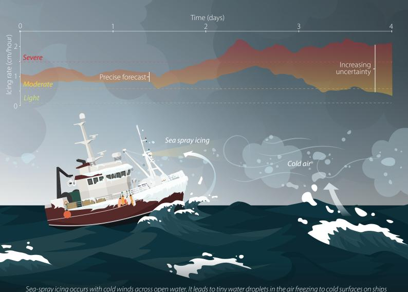
or other structures and forming a layer of ice. This accumulation can affect the performance of equipment and, in the worst-case scenario, the capsizing of the vessel.
