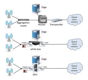
Fig. 1: Traditional optical network scenario with aggregation routers and standalone transponders (top); Evolved scenario with white box and coherent transceivers (center); innovative optical metro network scenario with edge computing nodes and DPUs with coherent transceivers (bottom).
