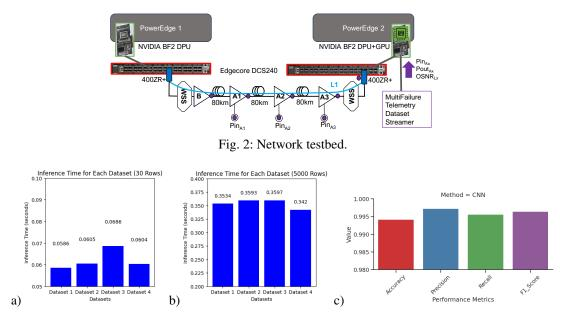
Fig. 3: (a)(b) Monitoring scenario Inference Time. (c) DDoS Attack Evaluation Results Using DPU.
