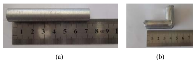
Fig. 2 Snap shots for sample (a) before and (b) after ECAP processing
