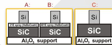
couple A: Si/h-BN spray (HeBoCoat 21E) coating/polycrystalline SiC
