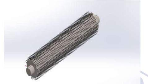
Figure 1. 3D view of a device that removes cotton fiber from saw teeth using a brush drum.
