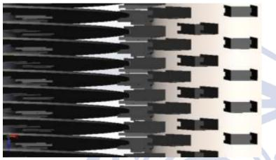
Figure 3. A view of a device that removes cotton fiber from saw teeth using a brush drum with a saw cylinder
