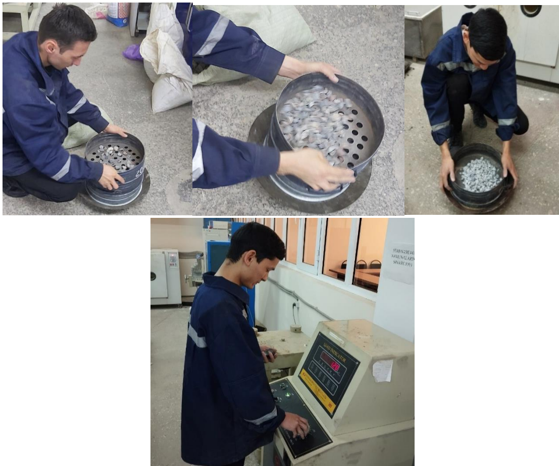
Figure 2: Crushed stone screening situation
