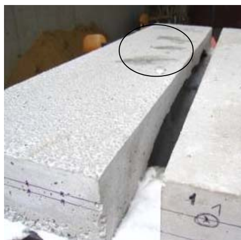
Fig. 3 Surface of the slab after thermal treatment – evaporation of water
