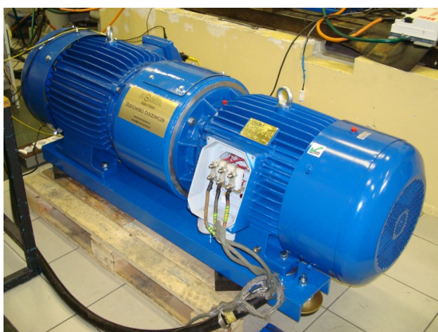
Fig. 21 Test stand of generator in special design in electrical machines laboratory of KOMEL
