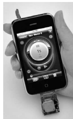
Fig. 2 The nanosensor device for cellphone integration and chemical sensing network [2]
