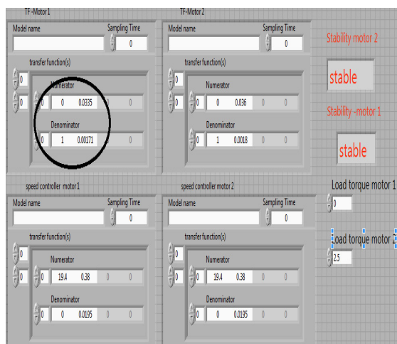
Fig. 7 Front panel representation for stability analysis of parallel connected induction motor drive for 25% increase in rotor resistance of motor 1
