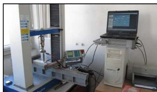
Fig. 2 Evaluation of electrical properties under loading
