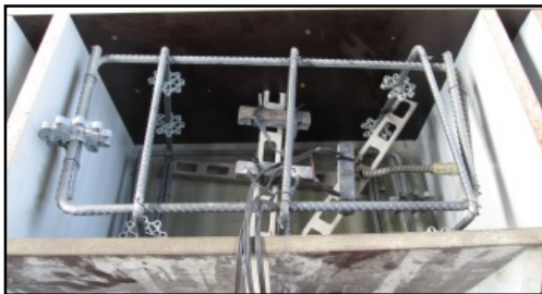
Fig. 4 Mold with the composite elements and steel reinforcement
