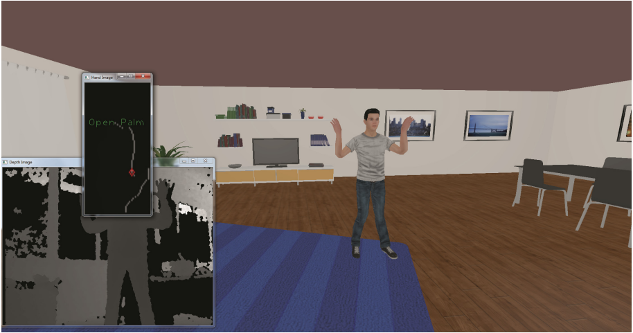
Fig. 4. Screenshot of an animated 3D avatar rendered by our Kinect full body avateering framework inside a virtual environment.
