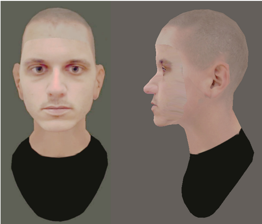
Fig. 7. Front and side view of real-time 3D facial animation avatar anchored at chin with body mesh. Post processing rendering effects are applied to ensure a smooth color transition between the face mesh and the body mesh diffuse textures.
