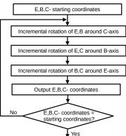
Fig. 2: Flowchart quaternion calculation
