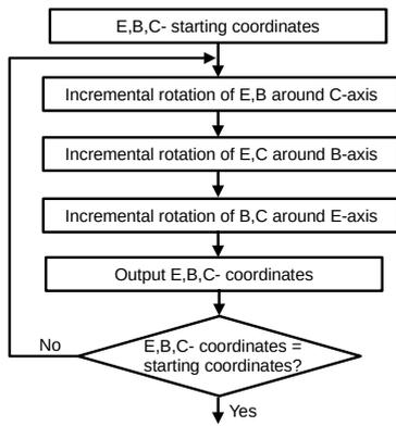
Fig. 2: Flowchart quaternion calculation
