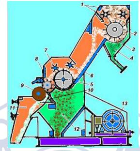
Fig. 1. Cross-section of the DV-1M roller gin.
