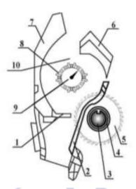
Figure 1. The working chamber of the saw demon
