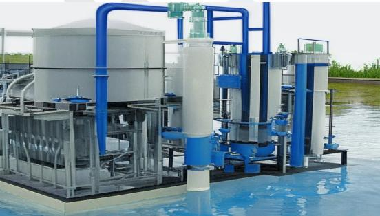
Figure 1. Ultrafiltration process for oily wastewater treatment
