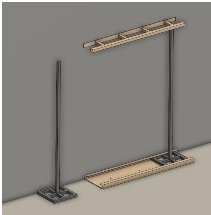
Figure 8: 3D-representation of the loading process. Bottles are stacked on the pole and slide into the rail
