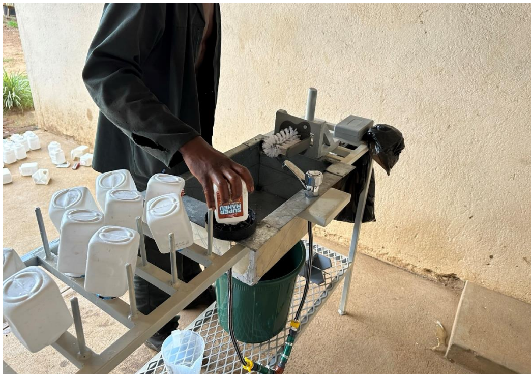
Figure 7: Cleaning Process of HDPE bottles. The vertical pins act as temporal storage of cleaned bottles.
