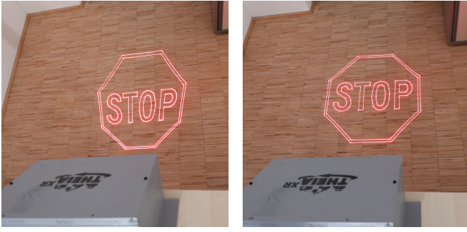
Fig. 4: (Left) A projected STOP sign appears distorted from the laser’s viewpoint after tilting the projector roughly 45°. (Right) The same sign appears undistorted after applying our oblique projection workflow.
