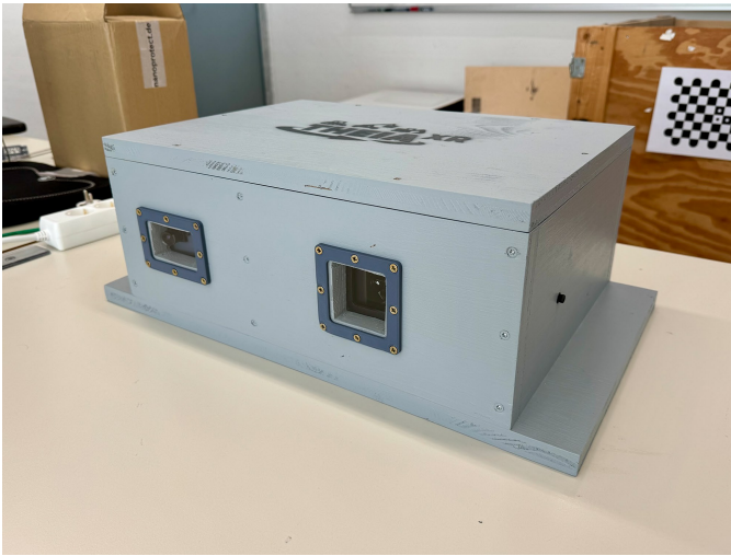
Fig. 5: (Left) Image of the proposed prototype with the camera aperture on the left side and the aperture for the laser projector on the right side. The baseline between both devices is 23 cm. (Right) Open prototype showing the internal components.
